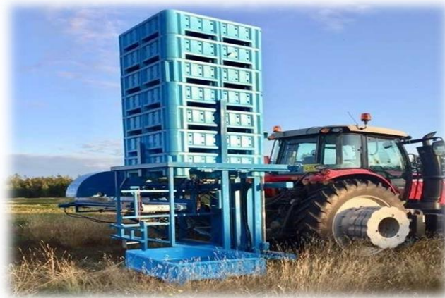
Figure 2: Semi-automatic bin handling system
