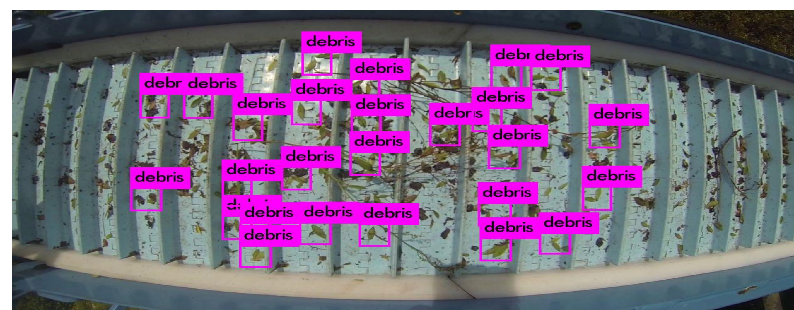
Figure 2: Debris detection using YOLOv3-Tiny
